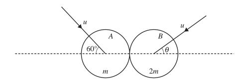
Two uniform smooth spheres A and B of equal radii have masses m and 2m respectively. The two spheres are moving with equal speeds u on a smooth horizontal surface when they collide. Immediately before the collision, A's direction of motion makes an angle of  $60^{\circ}$  with the line of centres, and B's direction of motion makes an angle  $\theta$  with the line of centres (see diagram). The coefficient of restitution between the spheres is e.
